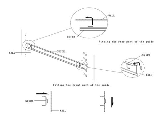
Reposition guide rail to the new location and reinstall in reverse order.
